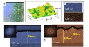
**Fig. 1**. TiO<sub>2</sub> sample grown under AW activation 2D pattern observed by the differences in topography (A), densification (B), and morphology and crystallinity (C).
